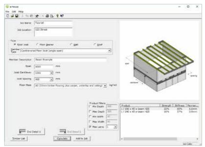
**HINT** The images on the right-hand side of the window show the user what member they are designing, as well as illustrating the required inputs, such as span, spacing and cantilever.
